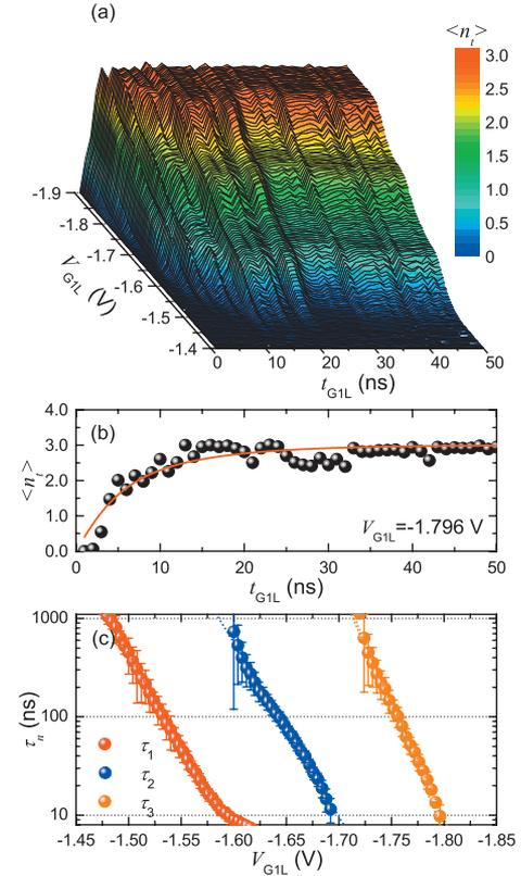
FIG. 2. (Color) (a) Average number of escaped electrons as a function of  $t_{G1L}$  and  $V_{G1L}$ . (b) Typical time-domain analysis at  $V_{G1L} = -1.796$  V. (c) Exponential dependence of the escape time on  $V_{G1L}$ . The bars show the standard error included in the fitting routine.
