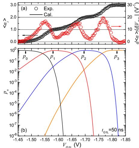
FIG. 4. (Color online) (a) Comparison of the experimental results with the calculated average number of escaped electrons and its first derivative with respect to  $|V_{G1L}|$ . (b) Escape probability of  $n$  electrons as a function of  $V_{G1L}$ .
