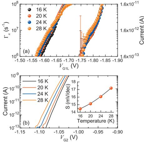
FIG. 3. (Color) Temperature dependence of (a) escape rate in the SE ratchet and (b) currents in the subthreshold regime of the MOSFET operated by G2 at  $V_D=100$  mV. In the upper panel (a), two series of plots show  $\Gamma_1$  and  $\Gamma_2$  from the left, and the right-side axis indicates the relevant current values. The inset in (b) shows the subthreshold swing ( $S$ -factor).
