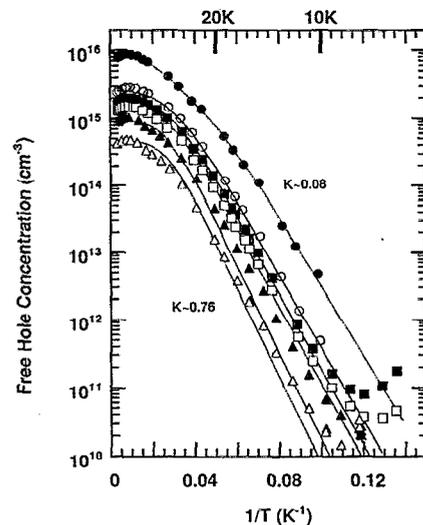
FIG. 1. Temperature dependence of the free hole concentration in samples B (●), C (○), D (■), E (□), F (▲), and G (△). Solid curves are fits obtained from Eq. (3).
