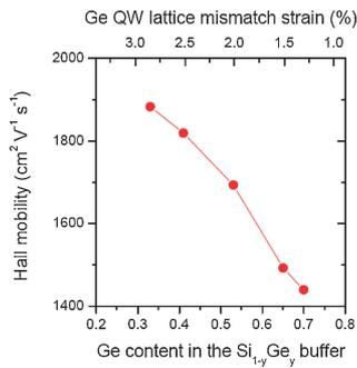
**Fig. 1.** Room-temperature Hall mobility of p-type MOD Si/Si<sub>1-y</sub>Ge<sub>y</sub>/Ge/Si<sub>1-y</sub>Ge<sub>y</sub>/Si(001) heterostructures as function of Ge content,  $y$ , in the relaxed Si<sub>1-y</sub>Ge<sub>y</sub> buffer and lattice mismatch between compressive strained Ge QW epilayer and relaxed Si<sub>1-y</sub>Ge<sub>y</sub> buffer layer. The data for samples with inverted doping and strain 2.5 and 2.9%, and samples with normal doping and strain 1.3–2.0% are shown.
