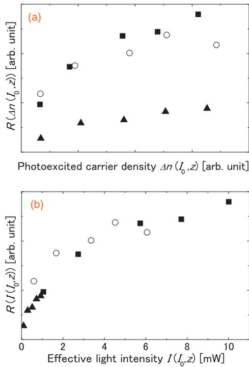
**Fig. 2.** Enhancement factor of the dislocation glide  $R(f(I))$  vs (a) photoexcited carrier density  $\Delta n(I_0, z)$  and (b) effective light intensity  $I(I_0, z)$  for three different dislocations situated at  $z \sim 1.0 \mu\text{m}$  (■),  $z \sim 1.7 \mu\text{m}$  (○), and  $z \sim 3.9 \mu\text{m}$  (▲) from the sample surface.
