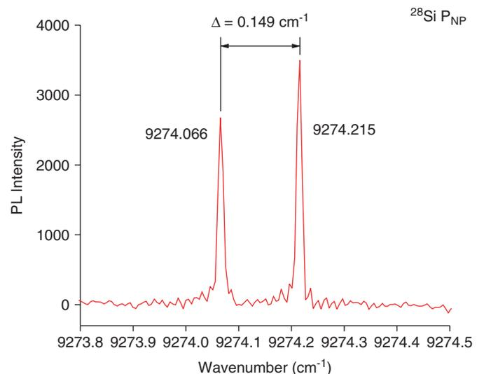
Fig. 2. PL spectrum showing the well-resolved splitting of the P BE NP transition in the  $^{28}\text{Si}$  epilayer in sample  $^{28}\text{Si}/^{nat}\text{Si}$  #2.
