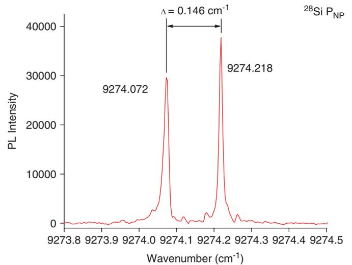
Fig. 1. PL spectrum showing the well-resolved splitting of the P BE NP transition in the  $^{28}\text{Si}$  epilayer in sample  $^{28}\text{Si}/^{nat}\text{Si}$  #1.
