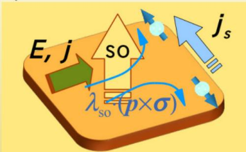
Coupling between spin and orbital motion by spin-orbit interaction
