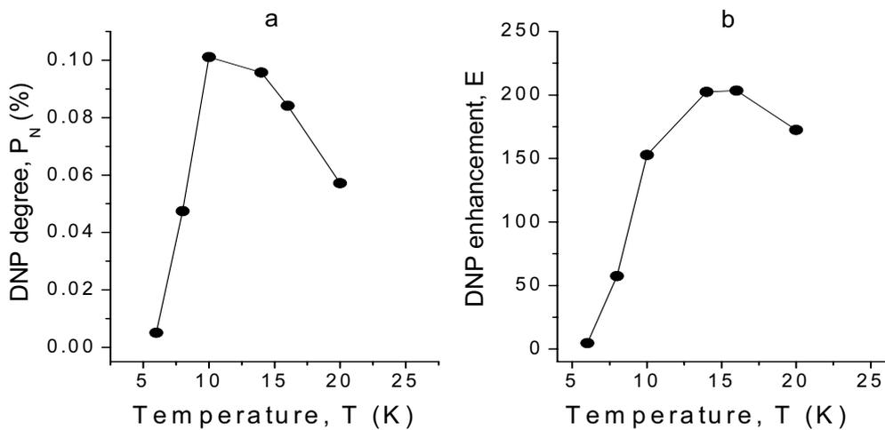
**Fig. 2** Dependences of the (a) degree of  $^{29}\text{Si}$  DNP,  $P_N$ , and (b) enhancement  $E$  on the temperature  $T$  in the naturally abundant silicon crystals.
