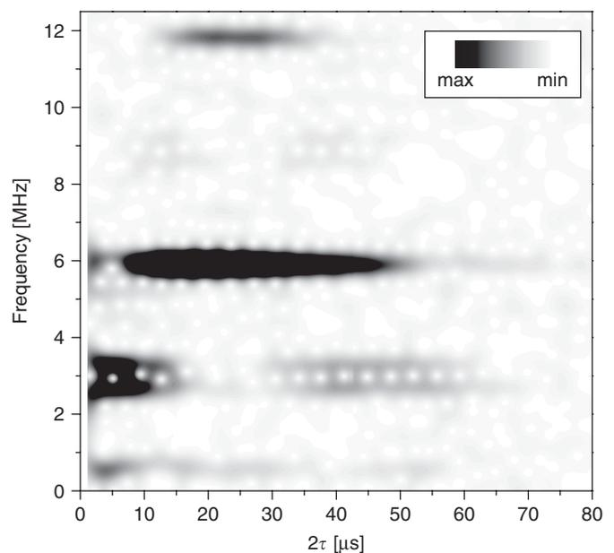
Fig. 3. Time-frequency space analysis of ESEEM in the sample with  $f = 99.2\%$  when the external field is applied along  $[001]$ .
