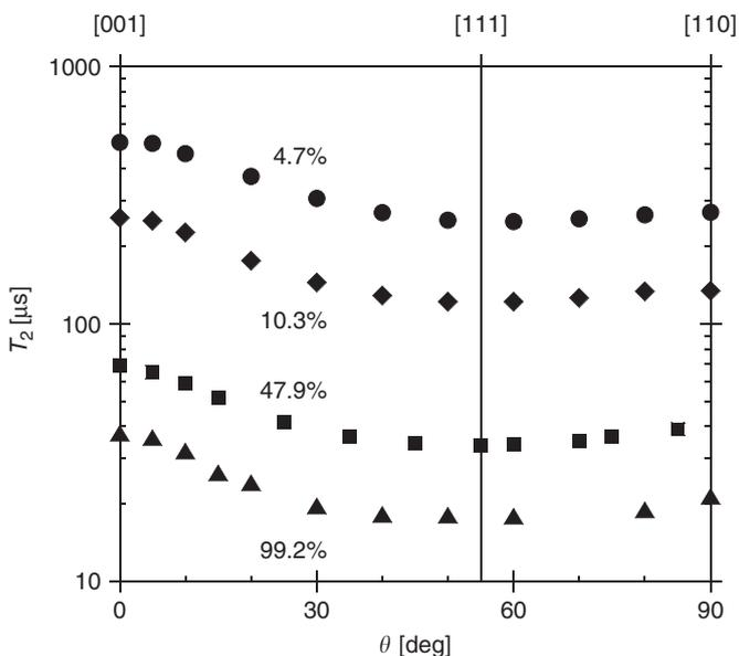
Fig. 2. Orientation dependence of  $T_2$ . Circles, diamonds, squares, triangles represent  $T_2$  for  $f = 4.7\%$ ,  $10.3\%$ ,  $47.9\%$ ,  $99.2\%$ , respectively.  $\theta$  is defined as the angle between  $B_0$  and  $[001]$ . See also Fig. 1(c).
